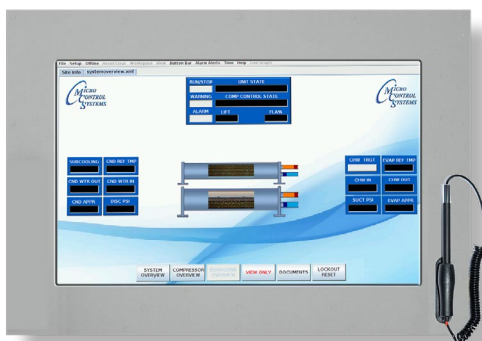
EVAPORATOR CONDENSER OVERVIEW SCREEN
